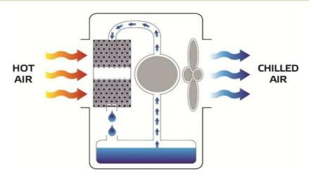
Master Bio Coolers cool the air using a simple natural process: the evaporating water decreases the temperature of the air. A pump takes the water from a tank and wets a wide filter of natural cellulose. A powerful ventilator aspires air through the filter. The water evaporates from the filter and decreases the temperature of the air of several degrees. The fresh and clean air flows into the ambient, and cools it.
