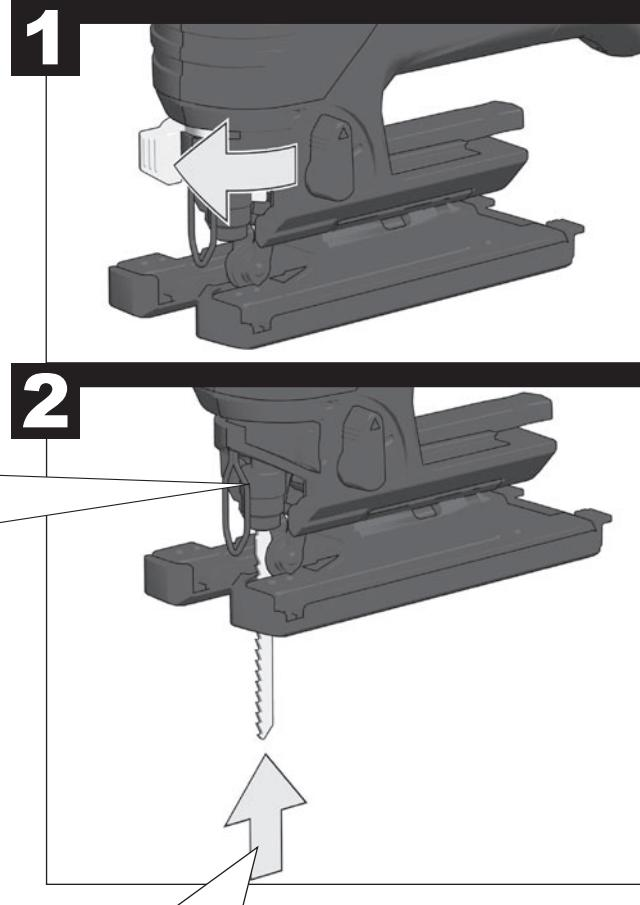
Press the saw blade into the Fixtec holder up to the stop.
