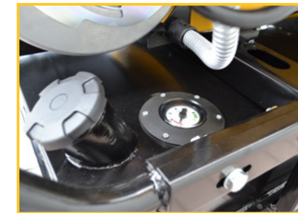
A leakless fuel tank closure and a big fuel level indicator
