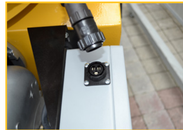
The motor is connected to the electronic panel with a snap-on connector, allowing an easy maintenance
