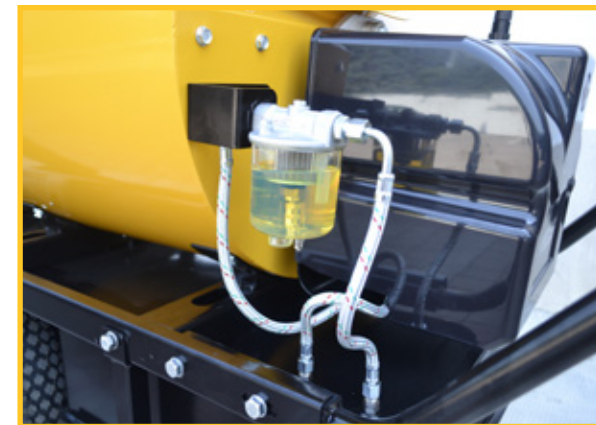
Dewatering unit: it eliminates water from the fuel. The fuel is then pre-heater within the combustion head
