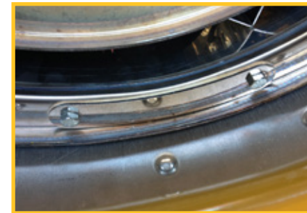
BV 500 has windows which allow an easy access to the heat exchanger for cleaning
